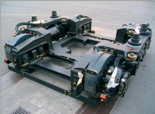
Fig. 4 El bogie motor SF 30 C TFW.
