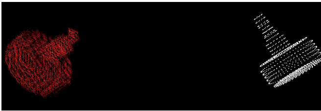
Fig. 3: The extractive results of the fiducial marker and of the point set of the model before registration
