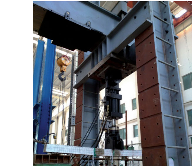
Fig. 2: Fatigue test and measurement. (a) Measurement. (b)Fatigue test
