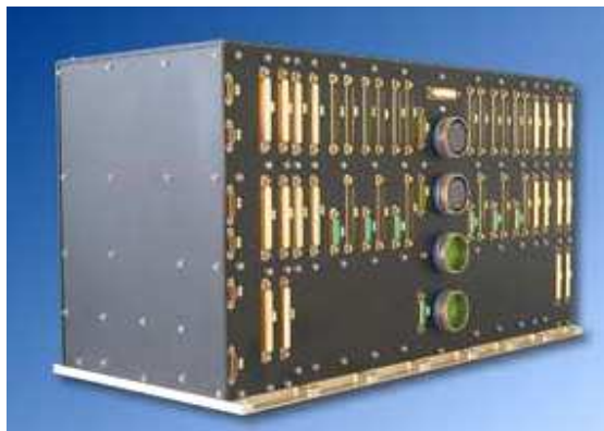
Fig. 12: Power control and distribution unit for the GOCE ESA satellite. Made in Crisa, Spain.
