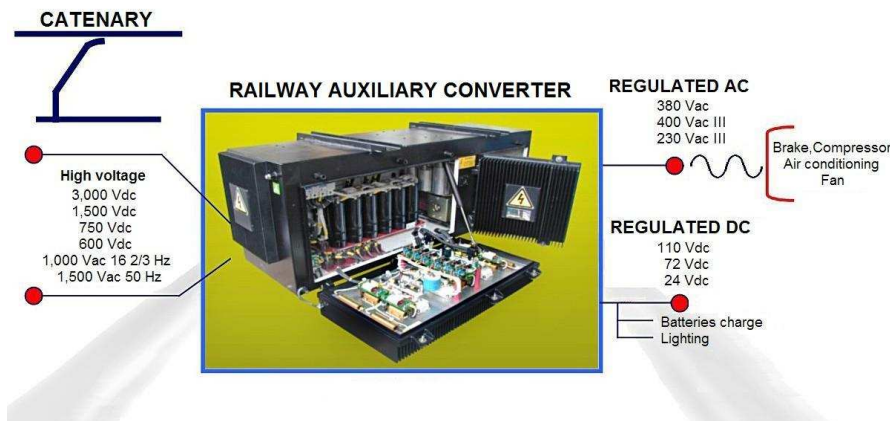
Fig. 7: Railway auxiliary converter. Input and output voltages. By courtesy of SEPSA, Pinto, Madrid.
