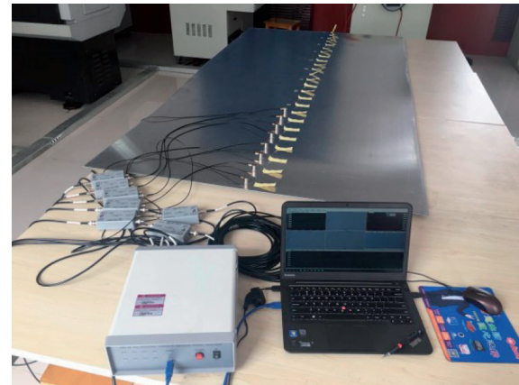
Fig. 3: Experimental system for the attenuation of acoustic emission waves
