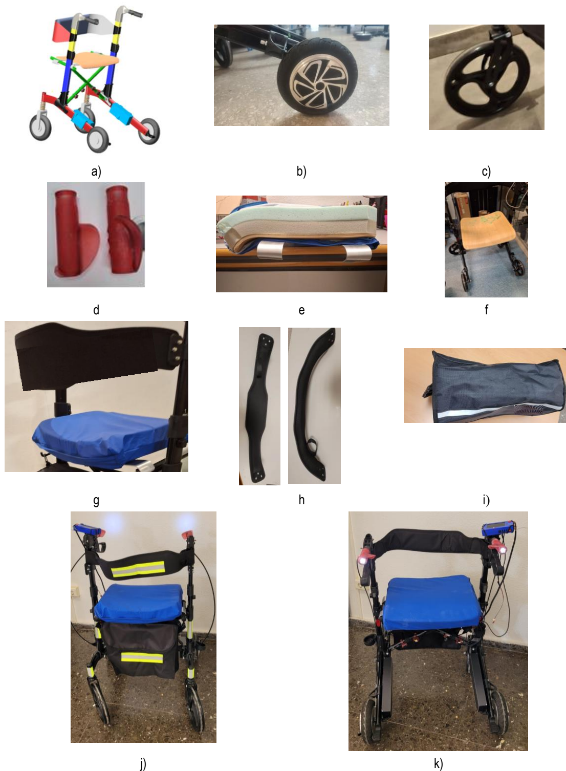
Figure 8. Robotic walker: a) 3D model, b) Rear wheel, c) Front wheel, d) Handles, e) Padding, f) Ergonomic base, g) Seat, h) Backrest, i) Basket, j) Front view of final walker, k) Rear view of final walker.
